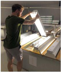
Figure 3. Charles Wilhelm removes a 3D color target from an accelerated fluorescent test unit.
