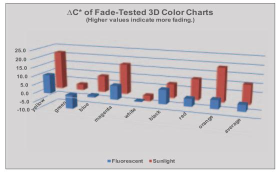
Figure 5. Graph of the change in chromaticity (C\*) of color patches exposed to fluorescent light and outdoor sunlight. The samples illuminated with sunlight (red) showed the greatest decrease in chromaticity due to light fading.
