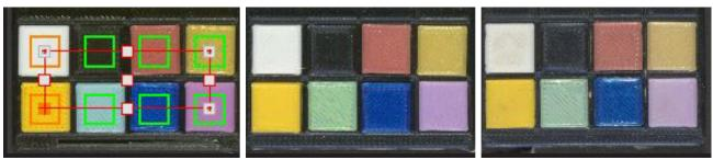
Photoshoot software measurement screen (green squares are the LAB measurement areas)
