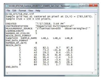
Figure 10. This CGATS standard file of LAB color readings is the output of the MegaVision Photoshoot software. The readings correspond to the 8 green rectangles in Figure 7.
