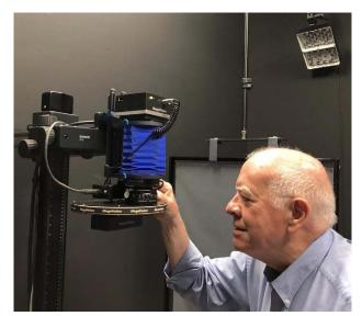
Figure 8. Henry Wilhelm adjusts the MegaVision EV Multispectral Camera. The EV is a spectral imaging system that employs a 50-megapixel monochrome CCD with a configurable LED array of up to 19 narrow-band LEDs (visible in upper right corner: UV 365, 385, and 400 nm; Visible 420, 450, 470, 505, 530, 560, 595, 615, 630, and 655 nm; and IR 700, 735, 780, 850, 940, and 1050 nm) in place of white light as the illuminant.
