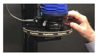
Figure 12. A closer view of the MegaVision EV camera showing the filter wheel that can be used to isolate selected wavelengths of illumination in order to quantify degradation of UV-excitation of fluorescing dye and pigment colorants. The filter wheel is also extensively used in the examination of cultural heritage objects.
