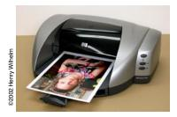
To switch the HP 5550 printer from the 4-ink plain paper mode to the 6-ink photo mode to print high quality, long-lasting photographs, the HP #56 Black ink cartridge is removed from the right-hand cartridge slot and replaced with the optional high-stability HP #58 Photo cartridge. The two cartridges can be easily changed back and forth.
