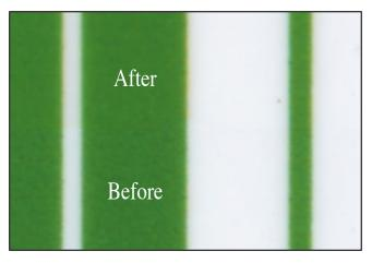
*Figure 4. Green/white color pair with line Bleed Rating = 1.0, "just noticeable bleed" (slightly softer edge was observed).*
