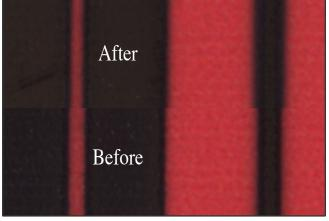
*Figure 6. Red/Black color pair with line Bleed Rating = 3.0, "very noticeable bleed."*
