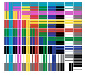
Figure 1. A line pattern test target of 36 color pairs (4 lines per color pair) for assessing image bleed in inkjet prints exposed to high humidity. 72 dpi line width.
