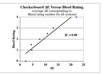
Figure 12. The correlation of  $\Delta E$  versus bleed rating number by pooling all data confirms that the rating was not system dependent.
